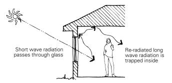
**Radiant heat** from the sun passes through glass and is absorbed by building elements and furnishings, which then re-radiate it. Re-radiated heat has a different wavelength and cannot pass back out through the glass as easily. In most climates, 'trapping' radiant heat is desirable for winter heating but must be avoided in summer.
