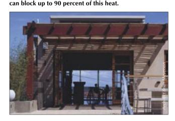
**Shading of glass** to reduce unwanted heat gain is critical. Unprotected glass is often the greatest source of unwanted heat gain in a home.
