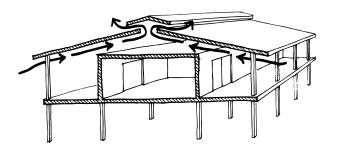
A 'fly roof' can be used to shade the entire building. It protects the core building from radiant heat and allows cooling breezes to flow beneath it
