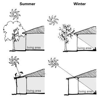
With ideal north orientation sun can be excluded in summer and admitted in winter using simple horizontal devices, including eaves. For situations where ideal orientation cannot be achieved (eg existing house, challenging site) it is still possible to find effective shading solutions. [See: Passive Solar Heating; Orientation]
